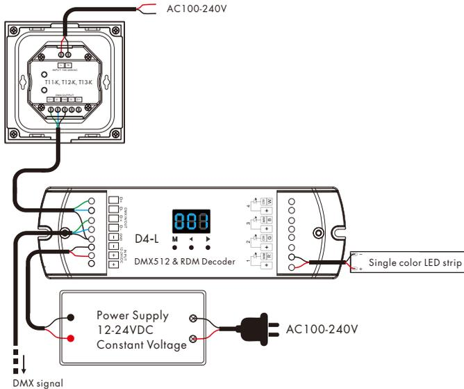
When the rotary panel controller work as DMX512 master, it can also match with the RF remote (optional). End user can choose the suitable match/delete ways. Two options are offered for selection:
