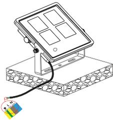
4. Switch mains power ON and test if light operates properly, using remote included, before finalizing the installation.
